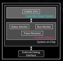
The on-chip debugger will monitor system busses, memory, CPUs, etc. Captured data will be used to extract useful features for analysis.
